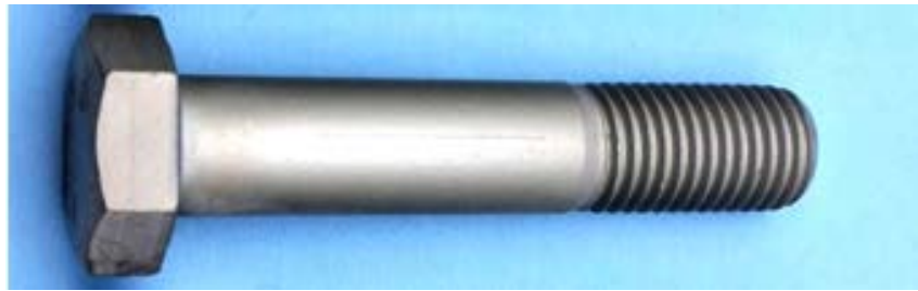
Figure 9 – Example of scribed bolt
