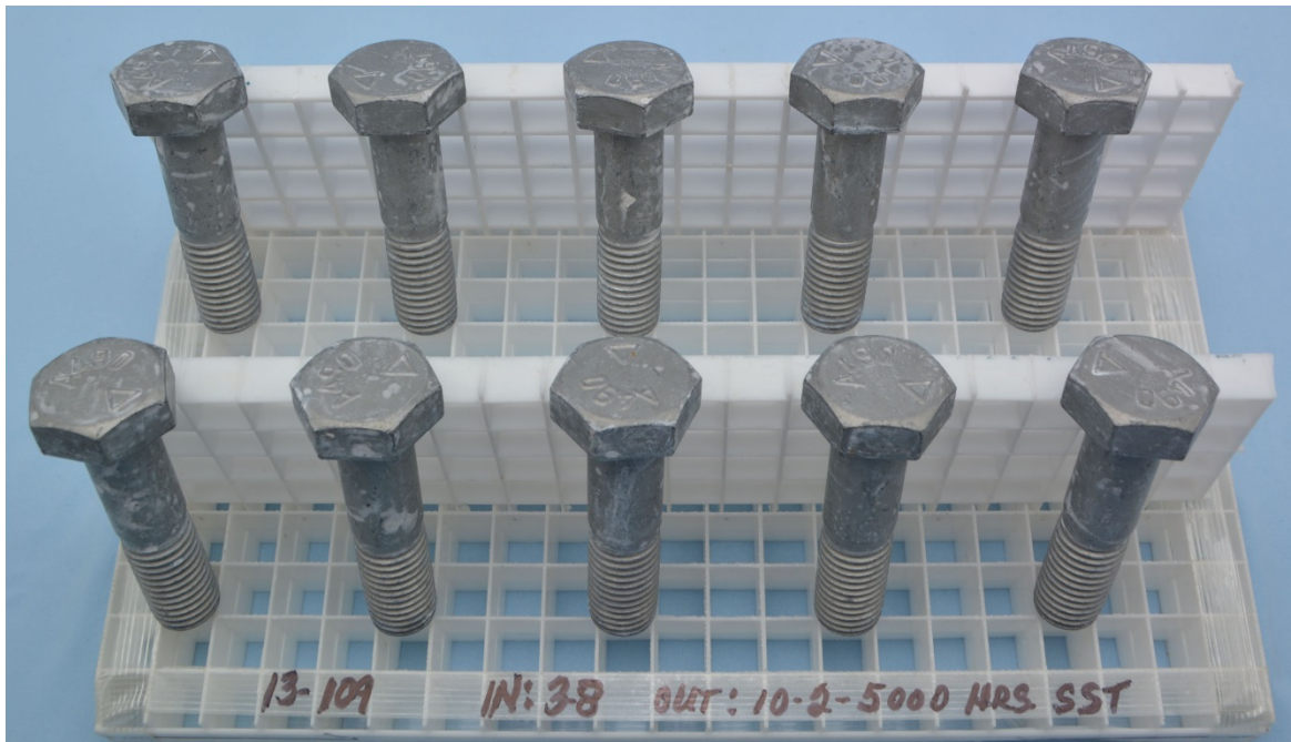
Figure 16 –3/4 inch bolts after 5000 h of salt spray exposure
