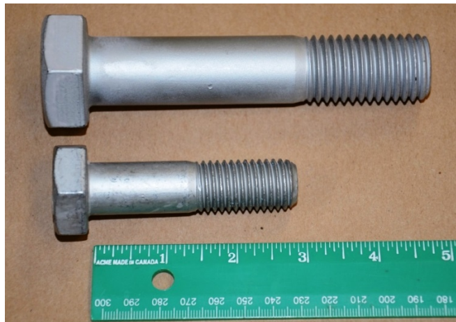
Figure 1 – Coated specimen bolts 1-8 x 5 and 3/4-10 x 3
